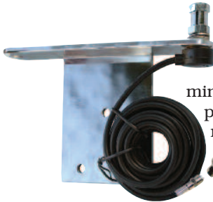
AUJ3K 1998-2006 Jeep external tail light mount, 8-1/2" polished aluminum, dual 1/2" hole mounting plate, 18' coax cable with weather resistant stud & quick on PL259. Enables mounting of two antennas or flag
